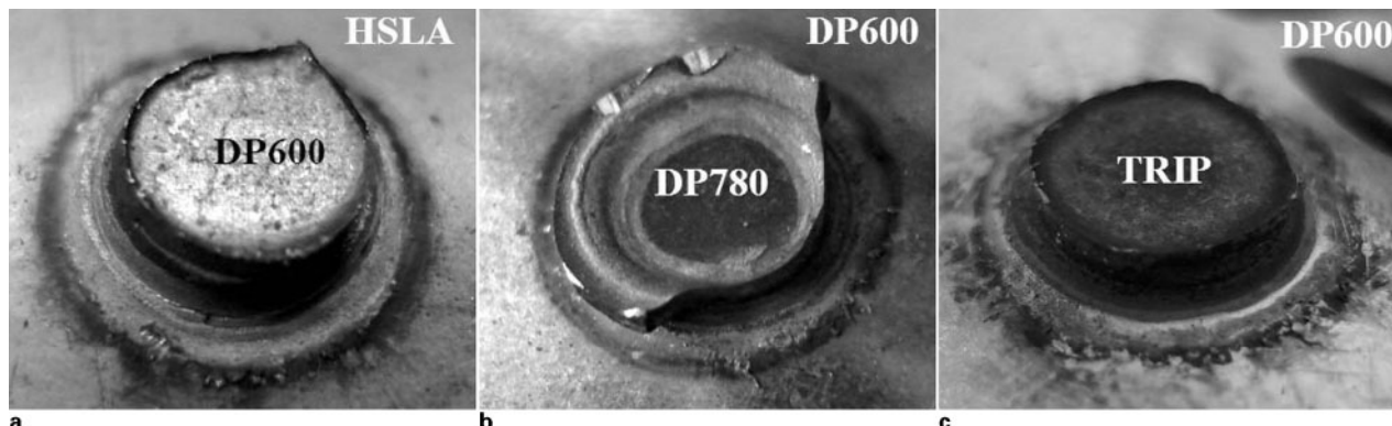
5 Cross-tension test failures
