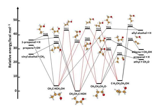
**Figure 1.** Simplified schematic diagram of the main reaction pathways in the dissociation of the 1-propanol radical. For clarity, the isomerization channels are depicted with red lines. Relative energies include ZPE contributions.
