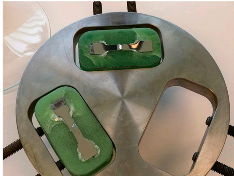
Figure A1. Specimens after polishing in Technovit-5071.
