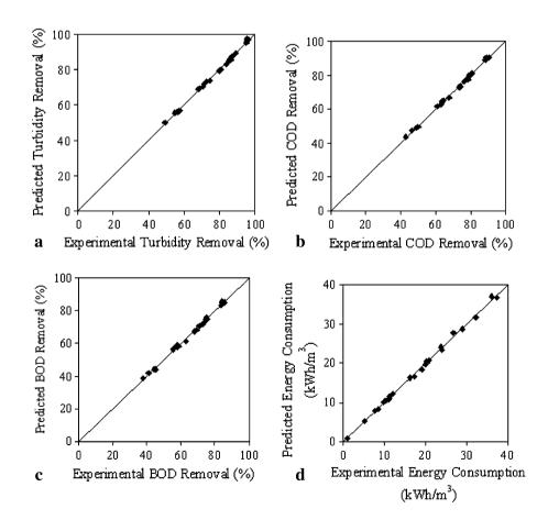
results for turbidity removal, COD removal, BOD<sub>5</sub> removal and energy consumption are shown in Table 4. The large value of F (604.85 for percentage turbidity removal, 397.76 for percentage COD removal, 377.19 for percentage BOD<sub>5</sub> removal and 147.59 for energy consumption) indicates that most of the variation in the response can be explained by the regression equations. The associated p value is used to estimate whether F is large enough to indicate statistical
