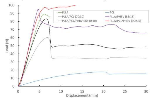
**Figure 4.** Representative load–displacement responses from filament tensile testing. **Table 3.** Mechanical properties for polymer filaments. Mean  $\pm$  s.d. *n* = 3.
