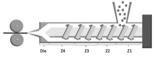
Figure 1. Schematic of extruder with temperature zones.
