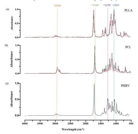
**Figure 3.** ATR-FTIR spectra for (**a**) PLLA, (**b**) PCL and (**c**) PHBV; the black lines are indicative of pre-extrusion and red lines of post-extrusion. Vertical lines indicate key wavelengths for ease of interpretation.
