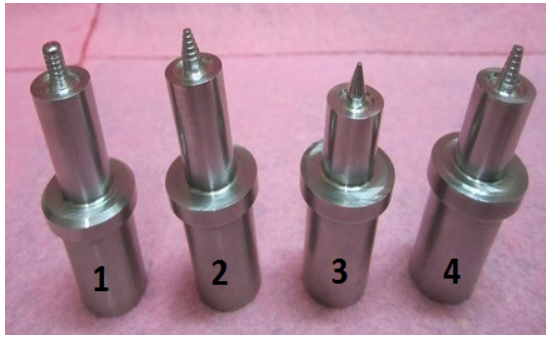
Figure 3. FSW tools with different pins and shoulders
