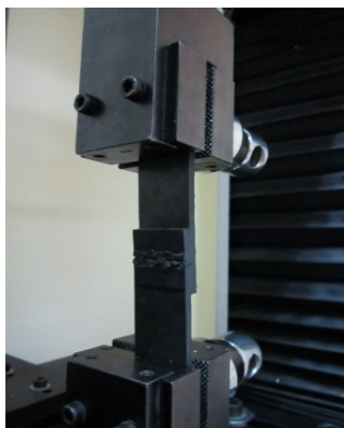
Figure 5. specimen during tensile shear strength testing
