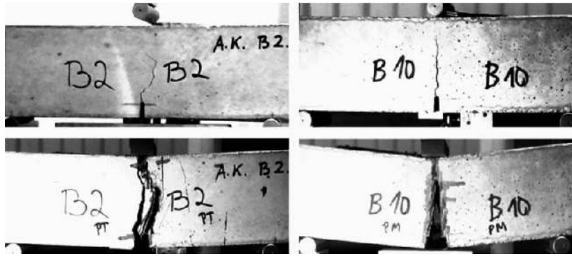
FIG. 4. Illustration of the damage in beams B2 and B10 (top: original beam, bottom: beam connected with polymer flexible joint) [6].
