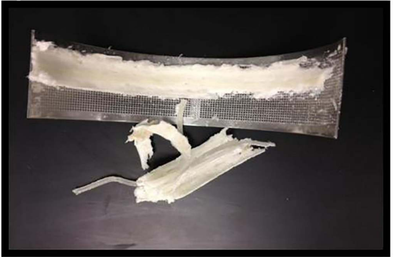
Figure 5. Failed milling of Klucel™ (ELF, EF, and LF) extrudates with PG injection.
