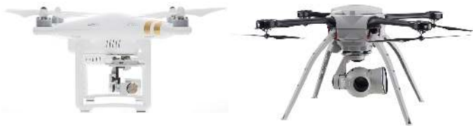
Fig. 4: Left: a multi-rotor with propellers in puller configuration. Right: a multi-rotor with propellers in pusher configuration.
