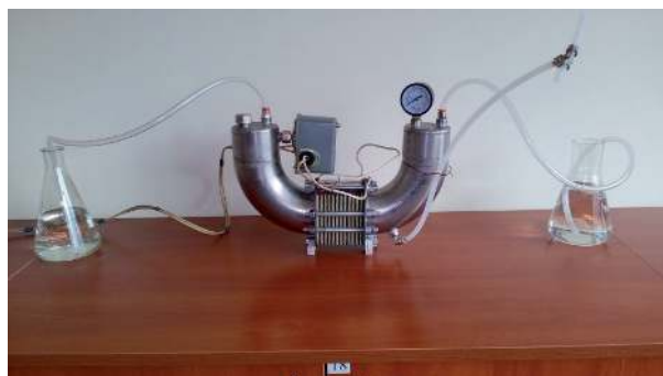
Fig. 2. External appearance of electric hydrogen generator H2-13B2
