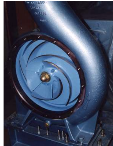
FIGURE 2: Pump with original impeller.
