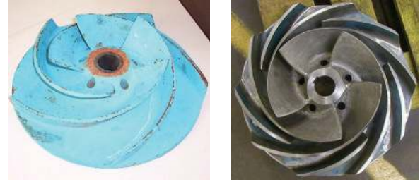
FIGURE 1: Original (left) and splitted (right) impellers.
