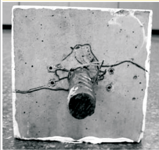
Figure 9 - Aspect of splitting cracks on the cross section
