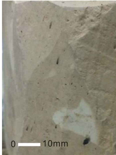
Fig.4. Photograph showing the meso-structure of the 20m loess
