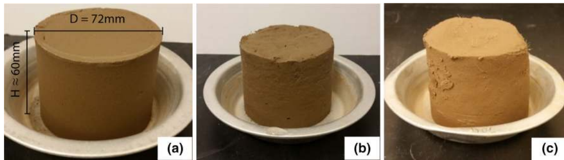
Fig. 8 PFT filter cake samples—no fibers (a), 18 mm fibers (b), and jute fibers (c)
