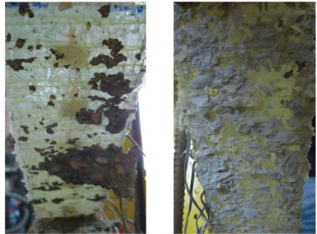
Fig. 11—Strips of 80 mm (3.150 in.). Failure surfaces after 3000 hours, 10,000 hours (7.5 and 47.5°C [45.5 and 117.5°F]) cycles.
