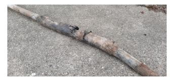
Figure 1. Example of damage to a cable joint mounted on a cable type XRUHAKXS  $1 \times 240/50$ .
