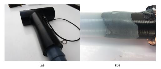
**Figure 3.** MV separable tee shape connector: (**a**) external view, (**b**) view of shield damage and control mantis deformation
