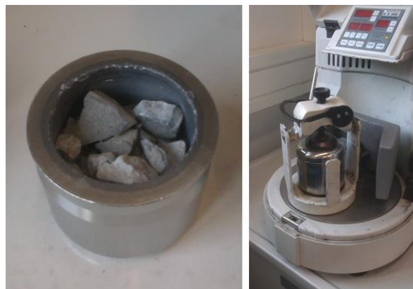
Figure 7: Slag sample preparation by milling in a ball mill
