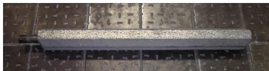
Figure 6: Pressed Ti-45Al electrode made from titanium sponge and aluminum rods
