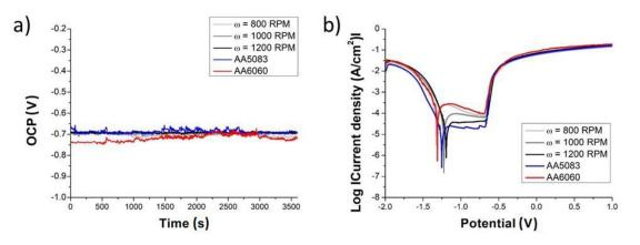
**Figure 10.** Open circuit potentials (*OCP*) (**a**) and potentiodynamic polarization curves (**b**) for all the tested samples in 3.5 wt% NaCl solution.
