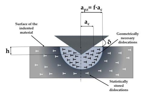
Figure 6. Cross-section of a sample during indentation tests.
