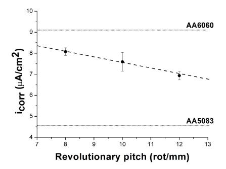
**Figure 11.** The relationship between corrosion current density (i<sub>corr</sub>) and revolutionary pitch for the produced welds.
