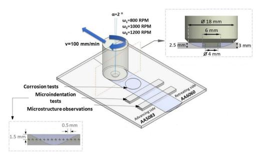
**Figure 1.** Schematic illustration of the process, geometry of the tool and location of the samples for the performed tests.
