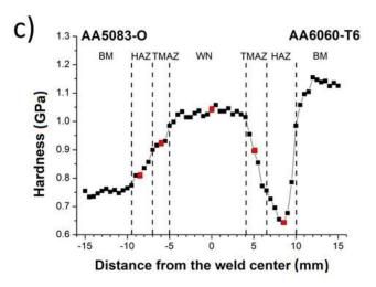
**Figure 4.** Hardness profiles of the joints produced with a tool rotational speed of 800 RPM (**a**), 1000 RPM (**b**) and 1200 RPM (**c**). Red dots indicate the exact locations of further dislocation density and mobility calculations.
