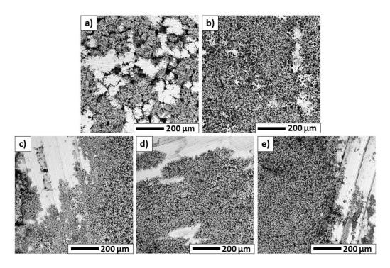
**Figure 12.** SEM images illustrating the surfaces of the samples after electrochemical tests on the base materials AA5083 (**a**), AA6060 (**b**), and the welds produced with tool rotational speeds of 800 RPM (**c**), 1000 RPM (**d**) and 1200 RPM (**e**).
