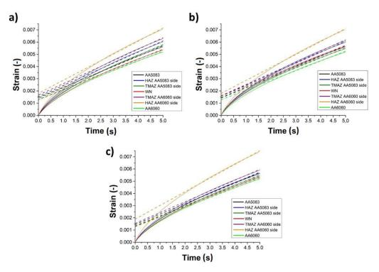
**Figure 8.** Strain versus time diagrams for the indentation dwell time period in the base metals AA5083, AA6060, HAZ, TMAZ and WN for the welds produced with tool rotational speeds of 800 RPM (**a**), 1000 RPM (**b**) and 1200 RPM (**c**).
