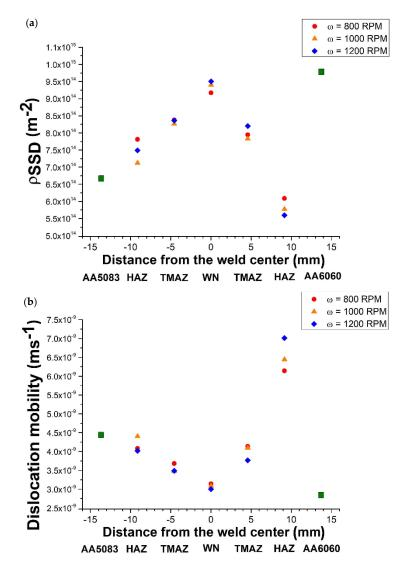
**Figure 9.** Density of SSDs (**a**) and dislocation mobilities (**b**) for all of the tested samples in different zones.
