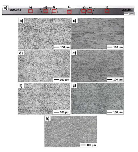
**Figure 3.** Macrostructure of the weld produced with a tool rotational speed of 1200 RPM (**a**), and microstructures of base metals AA5083 (**b**), AA6060 (**c**), HAZ on AA5083 side (**d**), HAZ on AA6060 side (**e**), TMAZ on AA5083 side (**f**), TMAZ on AA6060 side (**g**) and the weld nugget (**h**).
