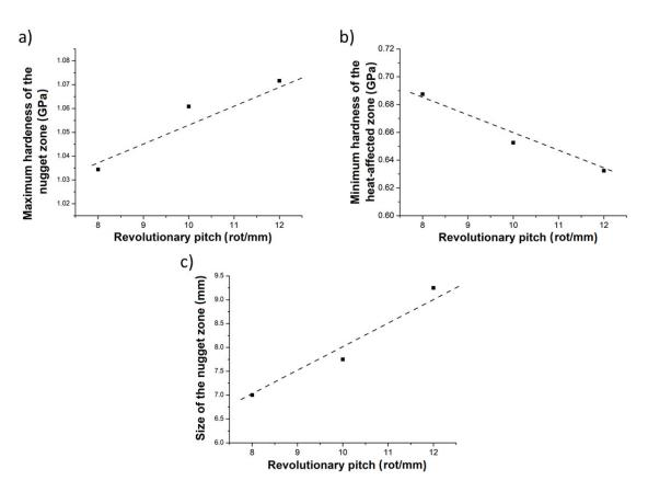
**Figure 5.** Relationship between the maximum hardness of the nugget zone and revolutionary pitch (**a**), minimum hardness of the heat-affected zone and revolutionary pitch (**b**) and size of the nugget zone and revolutionary pitch (**c**).
