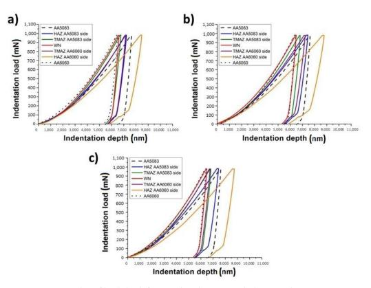
**Figure 7.** Hysteresis plots of load–depth for a single indentation in the base metals AA5083, AA6060, HAZ, TMAZ and WN, for the welds produced with tool rotational speeds of 800 RPM (**a**), 1000 RPM (**b**) and 1200 RPM (**c**).
