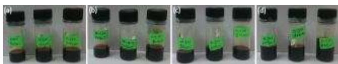
Fig. 1 Photograph of prepared ionic liquids (a) DMImI, (b) PMImI, (c) BMImI and (d) HMImI containing electrolytes.
