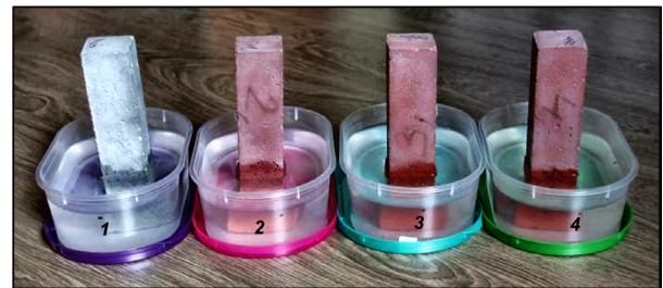
FIGURE 20. Risk of efflorescence in the pigmented alkali-activated slag cement mortars vs. the whitening additive: 1– reference sample (without additive); 2 – \text{TiO}_2 (5% by mass); 3 – kaolin (15% by mass); 4 – \text{CaCO}_3 (24% by mass). Content of pigment in mortar specimens (5% by mass).
