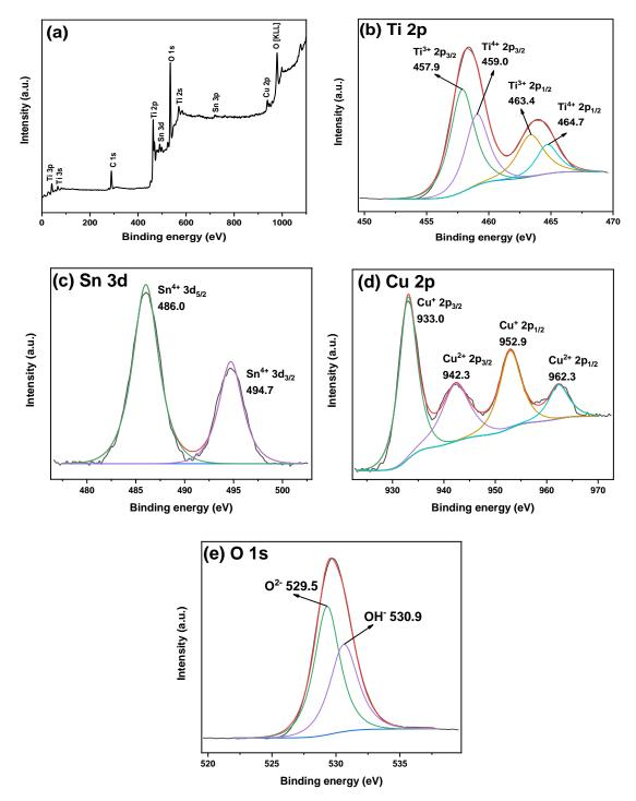
*Fig. 5. XPS spectrum of SCT: (a) total spectrum; (b) Ti 2p; (c) Sn 3d; (d) Cu 2p; (e) O 1s.* **3.4. Optical property**
