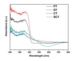
Fig. 7. Ultraviolet-visible absorption spectra of samples.
