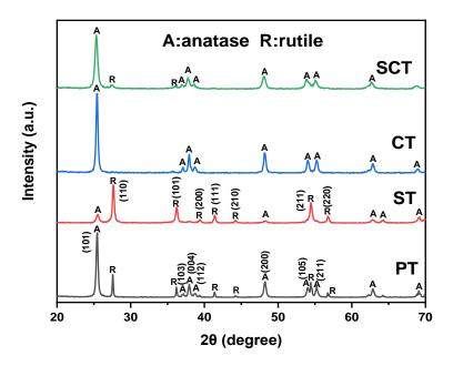
Fig. 1. XRD patterns of samples.
