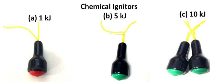
Figure 4: Chemical ignitors used in this work: (a) 1 kJ (b) 5 kJ and (c) 10 kJ
