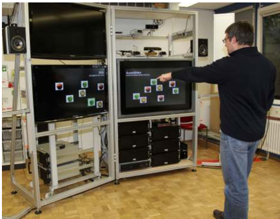
Figure 2: A user in front of the test system performing a selection using a pointing gesture
