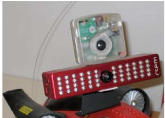
Fig. 1: Conventional pinhole camera aligned with Swiss Ranger
