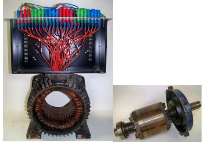
Fig. 6. 11kW induction machine modified to create faults by short circuiting coils. This machine allows one to make a minimal 12.5% of each phase coils in short-circuit.
