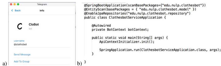
Fig. 17. a) A created chat bot and b) class ClothesbotServiceApplication with the main method
