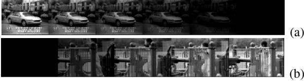
Fig. 1. Consecutive frames from “news” video sequence showing: (a) a fade-out; (b) a fade-in.
