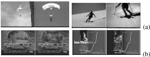
Fig. 12. Consecutive frames from video sequences presenting abrupt cuts, which caused missed shot cut detection: a) shot changes between two images with very similar spatial color distribution and b) shot change occurs only in a part of the video frame.
