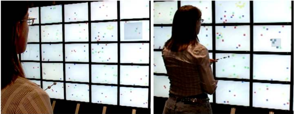
Figure 6: Using a wand to select at different scales based on distance from the display.
