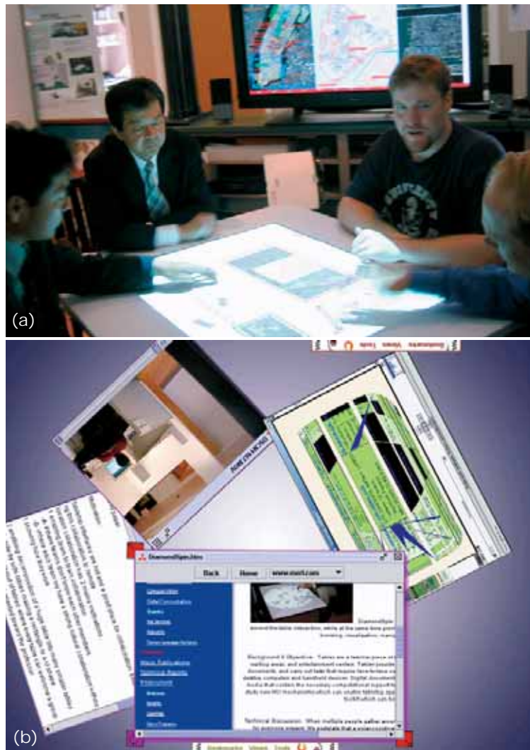
1 Content orientation in DiamondSpin Tabletop Toolkit. (a) Users meet around a multitouch, multiuser interactive digital table. (b) A bird's eye view of a DiamondSpin application, which constrains documents to face the tabletop's outside edge.
