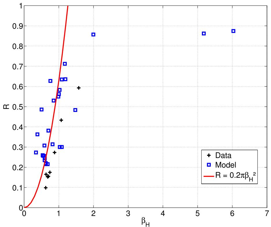
Figure 6: Relations between the reflection coefficient  $R$  and the normalized bed slope parameter  $\beta_H$ , modified from Van Dongeren et al. (2007)
