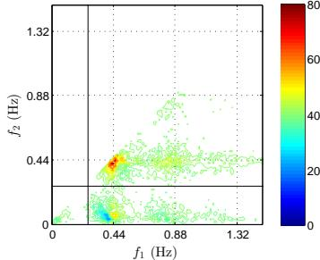
Figure 17: Imaginary part of the bispectrum in  $m^3 \times 10^{-8}$  of the incoming wave signal ( $\eta^+$ ) over a 1:80 laboratory slope, at  $x = 70$  m,  $h = 0.18$  m. Black solid lines indicate the cutoff between infragravity and sea-swell wave frequencies,  $f_{IG}$ . Dashed lines indicate the spectral peak ( $f = 0.44$  Hz) and its higher harmonics. After De Bakker et al. (2015a).
