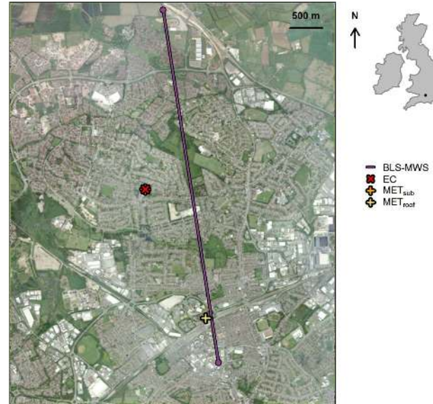
Figure 1. Aerial photograph (2009, GeoPerspectives © ) of the study area showing the locations of the two-wavelength scintillometer path (BLS–MWS), eddy covariance station (EC) and two meteorological stations (MET sub , MET roof ). The location of Swindon within the British Isles is shown (top right panel).
