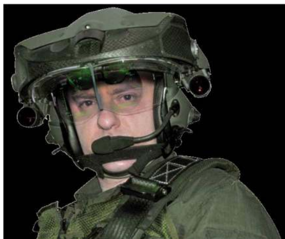
Fig. 16. Tales TopOwl® helmet incorporate an optical combiner assembly for each eye, allowing the pilot to view the cockpit and the outside world directly with the night imagery superimposed on it. TopOwl® has a 40° FOV and a total headborne weight of 2.2 kg in full configuration. Reproduced from [16].
