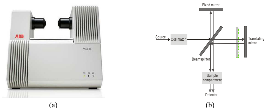
Fig. 39. The ABB MB3000 Series FT-IR Laboratory Analyzer: (a) photo and (b) schematic block diagram ( http://www.abb.com ).
