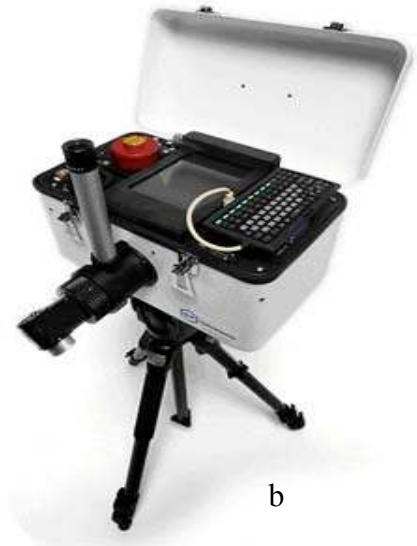
Figure 3 (a) Schematic diagram of the model 102F portable FTIR by Design & Prototypes, LTD; (b) Snapshot of the instrument.
