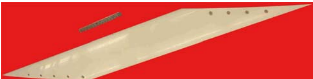
Fig. 1 Aluminum, powder coated model. Flow from left to right . 73^\circ leading-edge sweep angle, 71.2^\circ trailing-edge sweep angle, 0.349 m streamwise root chord, 0.271 m streamwise tip chord, 0.304 m streamwise mid-span chord, t/c = 4\% . Model mounted on C -channels
