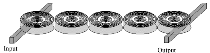
Fig. 5. Illustration of ABR-based CROW employing a vertical coupling scheme to conventional waveguides.
