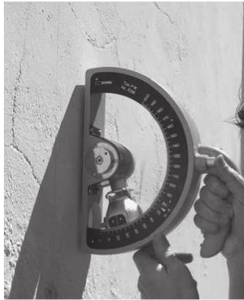
Figure 11: Pendular Schmidt impact hammer test.
