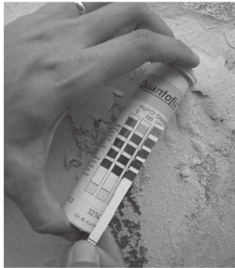
Figure 10: Strip tests – semi-quantitative determination of salts.
