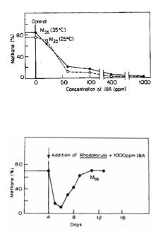
**Figure 2.** Inhibition of methane formation by IBA in M-25 and M-35 grown on acetate. Total incubation time - 2 days. Temperature of incubation was 25°C for M-25 and 35°C for M-35. Average concentration of IBA in a digester operating at ambient temperature varies between 40-60 ppm.
