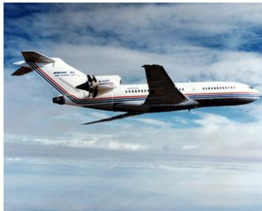
Figure 2. Rear-mounted open rotor pusher configuration, shown on Boeing 727 test vehicle.
