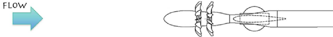
Figure 5. F31/A31 open rotor test article and linear microphone array in the NASA Glenn 9- by 15-ft Low Speed Wind Tunnel (Diagram courtesy of Edmane Envia, NASA Glenn Research Center).
