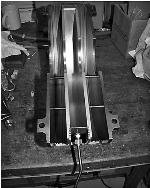
Fig. 4: Shroud before installation in test facility, showing adjustability of clearance radially and axially.
