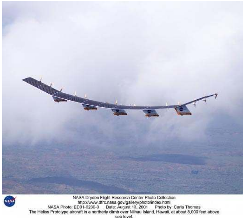
Figure 3 Helios High Altitude Long Endurance Solar Powered UAV
