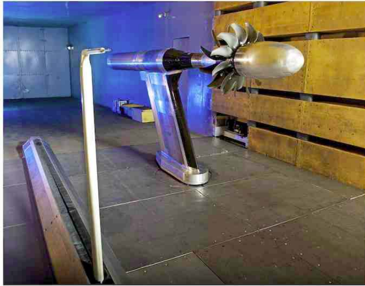
Figure 2.—The open rotor propulsion rig and traversing microphone probe installed in the NASA Glenn 9- by 15-Foot Low-Speed Wind Tunnel.
