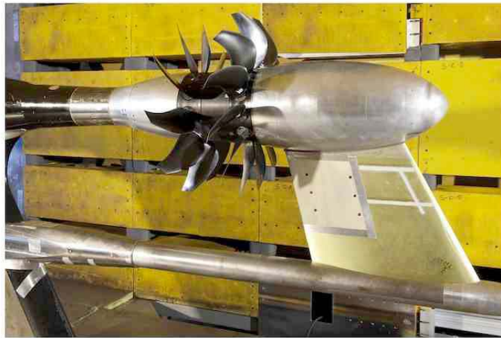
Figure 3.—The open rotor propulsion rig installed in the NASA Glenn 9- by 15-Foot Low-Speed Wind Tunnel with pylon hardware mounted.
