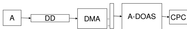
Fig. 4. A flow diagram of experimental setup used to measure the optical properties of a monodisperse PSL sample with the AE-DOAS. A = atomizer, DD = diffusion dryer, DMA = differential mobility analyzer, AE-DOAS = aerosol extinction differential optical absorption spectrometer, which is shown in detail in Fig. 2, and CPC = condensation particle counter. Additional instrument details are given in the experimental section.
