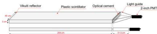
Fig. 7 A schematic view of a muon detector
