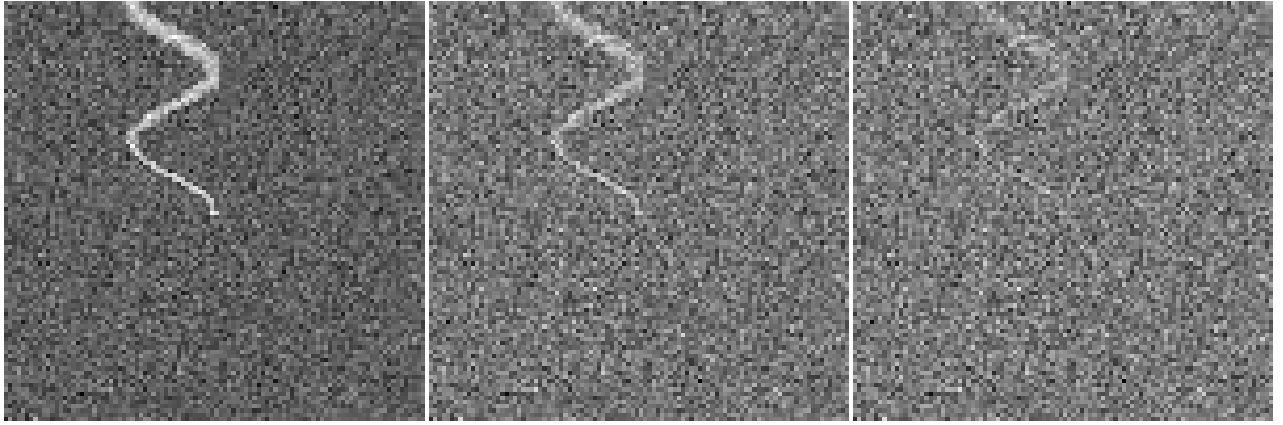
Fig. 6. A slice ( x -vs- z at y=50 ) along the center of the tube in the simulated data with three different levels of Gaussian noise added. Noise standard deviations are ( Left ) \eta=20 , ( Middle ) \eta=40 , and ( Right ) \eta=80 . The tube's noise-free, cross-sectional intensity profile is shown in Fig. 5.
