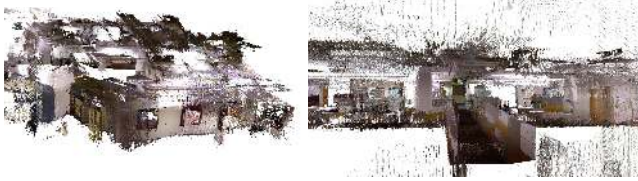
Fig. 5. cubicle: Reconstruction obtained by aligning the 3D laser scan in a global map, using the pose estimate from chord+gtsam (1 iteration).
