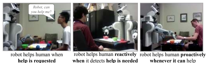
Fig. 1. Different initiative models for robot assistance during collaborative task executions: human-initiated help (left), robot-initiated reactive help (middle), and robot-initiated proactive help (right).
