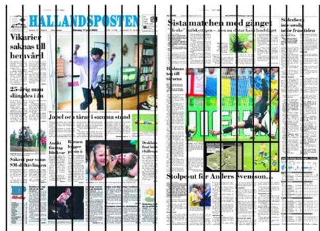
Fig. 3 An example of how the ink zones subdivide the paper fold
