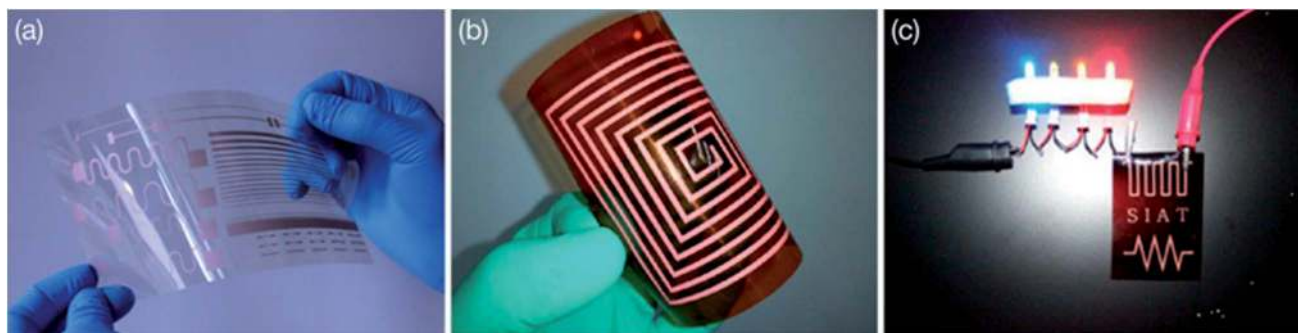
Fig. 31 (a) Photograph of inkjet-printed highly conductive copper patterns on a flexible poly(ethylene naphthalate) (PEN) substrate after plasma treatment. [Reprinted with permission from ref. 271 Copyright © American Chemical Society.] (b) Photograph of the copper-conductive-ink-based printed pattern on a flexible polyimide substrate. (c) Lighted LED device connected with the copper-printed circuit board. [Reprinted with permission from ref. 272 Copyright © American Chemical Society.]
