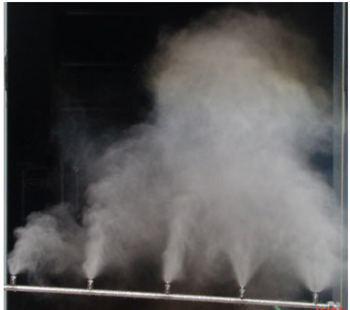
Figure 5. Various impaction-pin nozzles, from 147-micron (on right) to 457-micron orifice diameter (left), operating pressure 138 barg
