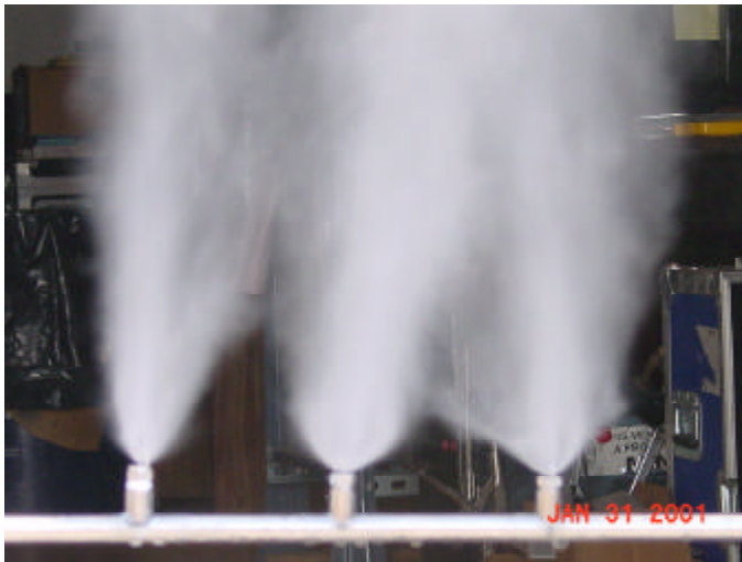
Figure 4. Visual plume shape of different makes of impaction-pin nozzles at an operating pressure of 138 barg (2000 psig). Mee nozzle (152 micron orifice, 316 stainless steel construction) in the center
