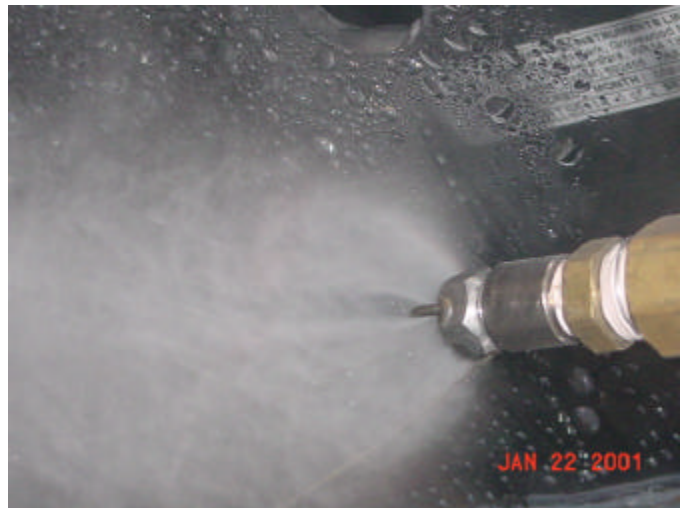
Figure 6. Impaction-pin nozzle showing small shading effect from impaction-pin
