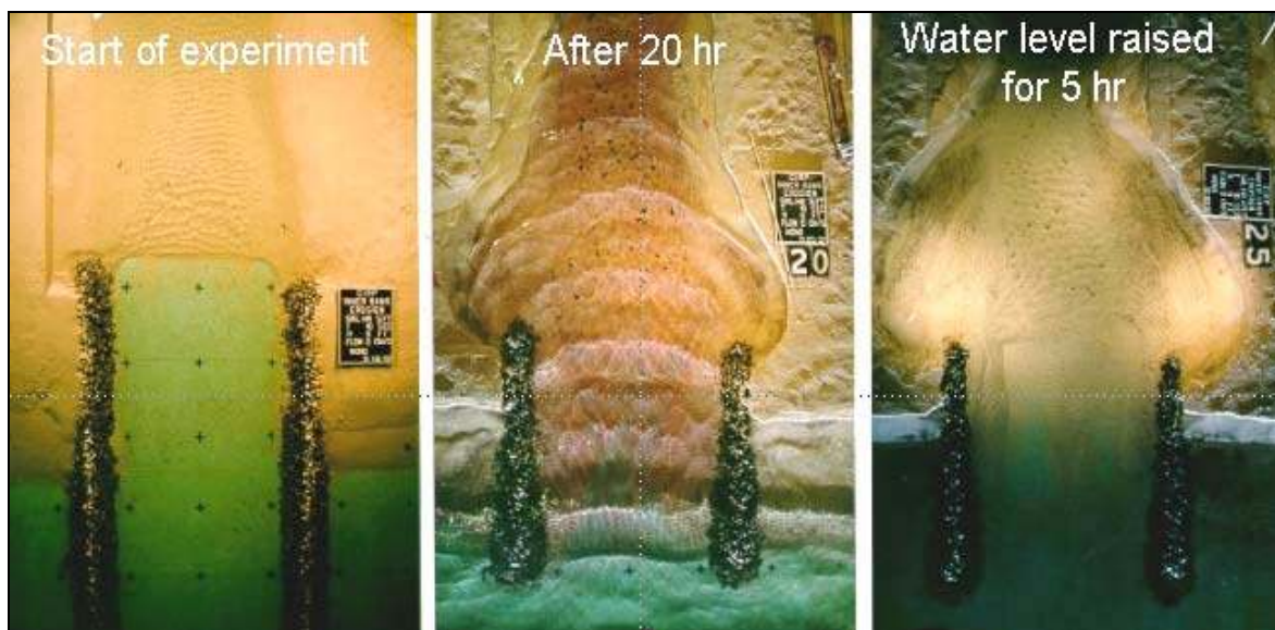
Figure 7. Physical model experiments showing inner-bank erosion development
